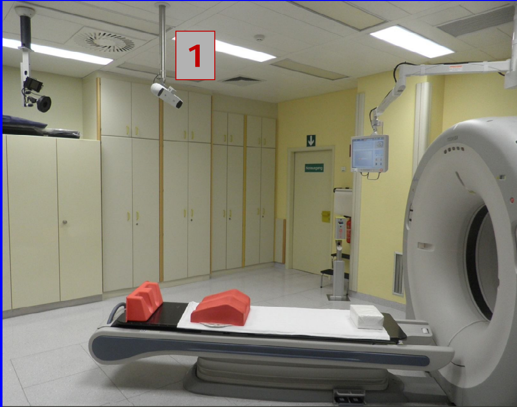
TOSHIBA Aquilion CT-simulator 1...infrared positioning, 2...CLARITY US-system
