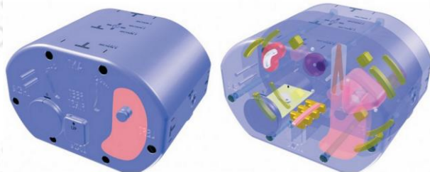
The DP-1000 is the most comprehensive "End-to-End" phantom that evaluates the entire radiotherapy process for Simulation, Treatment Planning, Imaging, and Delivery, including TG-53, TG-66, and TG-142.
